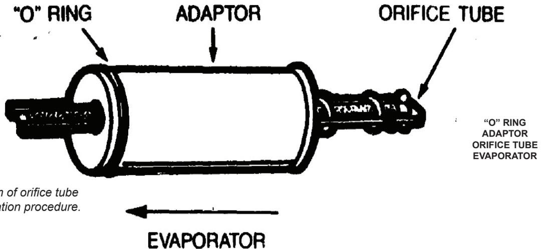
Figure 1. Diagram of orifice tube adapter kit installation procedure.
