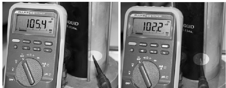
Temperature of Bare Metal and Painted Surface of Heated Charging Cylinder Measured with Contact Probe– Only Few Degrees of Temperature Difference
