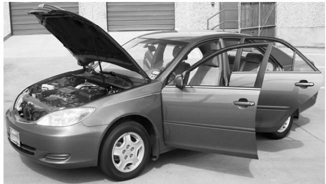
The Maximum Heat Load Temperature Test Is Performed Outside, In Direct Sunlight with Doors & Windows Open
