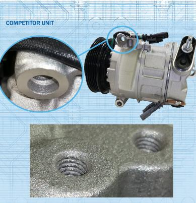
The competitor unit shows signs of sandblasting of the threaded surface. This lack of process control creates a coating that could cause the thread wall to strip, making installation difficult.
