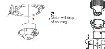
Re-use cap..lnsert new motor, add adaptor ring using screws supplied in kit, insert back into case.
