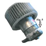
Four Seasons developed a protruding vent tube design that helps stop the water from flowing into the motor.
