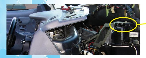
Air door actuators located behind the dash require full removal and up to eight hours of labor.
