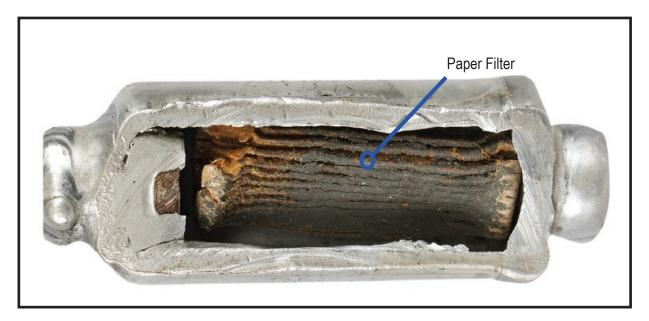
GM has recently added an in-line filter (pictured above) to the discharge hose on many vehicles. The filtering material is a paper product, which looks very similar to the in-line fuel filter used on many GM carburetors. However, this filter is not serviceable.
