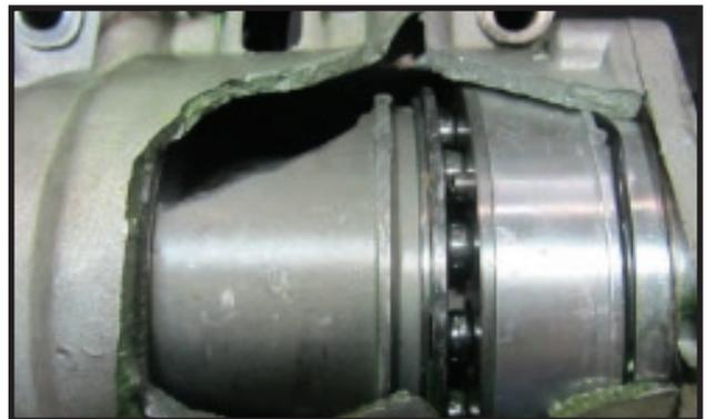
Lubricant stops moving and the compressor fails.
