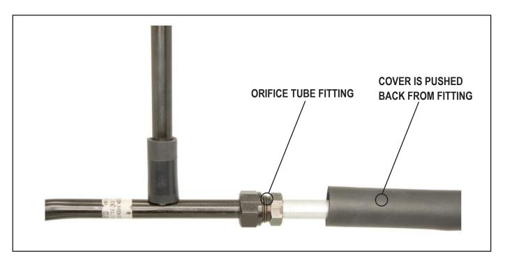
The fitting is covered with a protective rubber cover. The cover makes it hard to see the fitting and that the orifice tube is replaceable.
