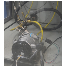
Four Seasons® compressors are performance tested on a calorimeter prior to being released to the production team.
