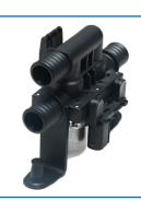
Commonly used on automatic temperature control (ATC) systems, this is a pulse width modulated (PWM) solenoid valve operated by the ATC control module. A second solenoid is used on dual zone systems. Other electronic heater valves use an electric rotary motor to control the coolant flow.
