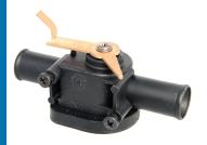
Normally used on systems without an air door actuator. The valve can manually be positioned from fully open (max heat) to fully closed (no heat) or anywhere in between (regulated heat).
