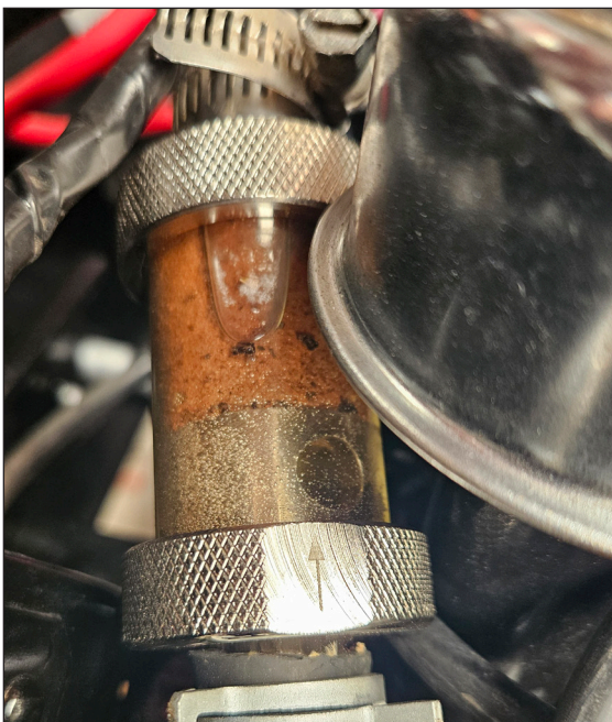
Debris caught in engine coolant filter that would have reached the heater core.
