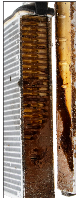
Heater core clogged with debris that could have been prevented with the addition of the engine coolant filter and resulted in complete heater core replacement.
