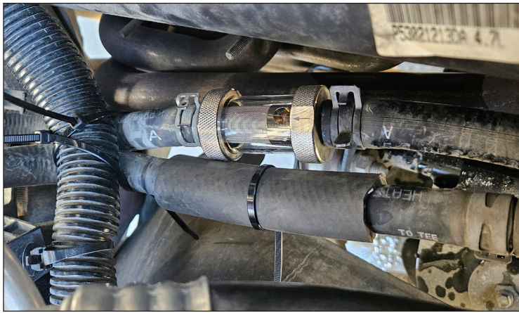
Engine coolant filter installed on a 2004 Dodge Ram pickup.
