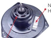
No Sealing / Protection of Heat Sink & Electronics
