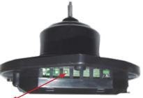
Exposed Traces on Printed Circuit Board (PCB)
