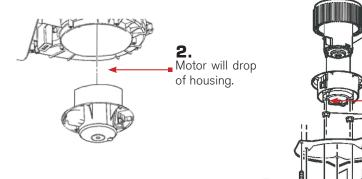
Re-use cap..lnsert new motor, add adaptor ring using screws supplied in kit, insert back into case.
