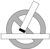
**LIMITATION**– A rigid probe can make solid contact difficult in hard to reach locations and tilting can alter readings as much as 20°F. Clamps can be hard to attach in tight spots without removing other parts for access.
