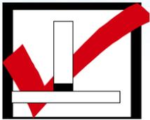
**ADVANTAGE**– More accurate temperature reading due to physical contact with component. For best results, the tip should rest squarely on the component. A clamp style pyrometer offers more consistent contact.
