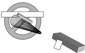
**LIMITATION**– Temperature readings can be affected by surrounding heat sources such as an exhaust manifold or radiator. Most infrared pyrometer's 'target area' increases with distance. Example: A one inch diameter 'target area' from six inches away can increase to a four inch diameter 'target area' twenty inches away. Also, some laser sights (red dot) may not point at the actual test location. The red dot could be a half-inch or more from the 'target area'.
