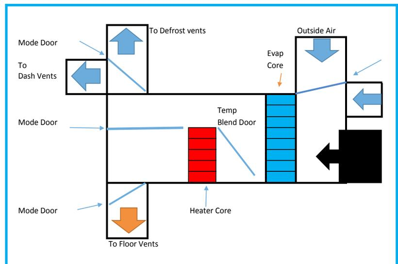
Materials being placed or collected in the system, most often occur when the vehicle has been parked for an extended period of time or is located in a rural area. Also Remember that many of today's vehicles utilize filter assemblies that have specific replacement intervals, which if overlooked can result in limited airflow.
