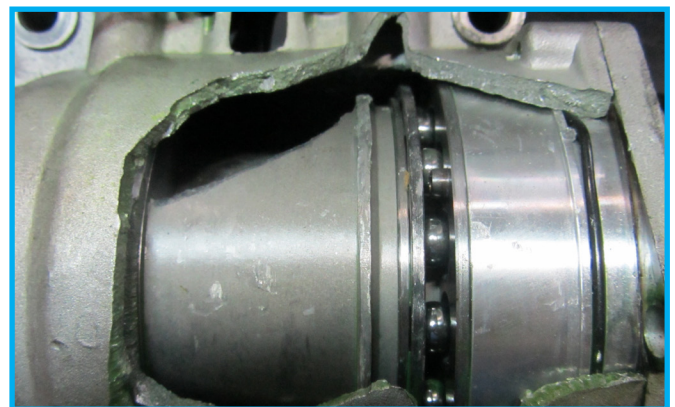
Lubricant stops moving and the compressor fails
