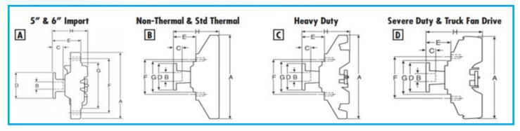
When disengaged, a fan clutch is designed to operate at 20 to 30 percent of the driven speed to help reduce the parasitic drain on the engine, increasing fuel economy. One of the primary differences between a Standard Duty, Heavy Duty, and Severe Duty fan clutch is the driven fan speed when engaged.
