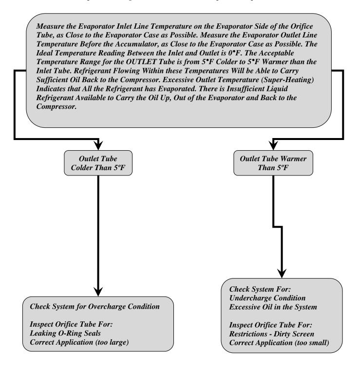
Note: Diagnostic Chart C applies to orifice tube systems. Most TXV systems do not provide easy access for superheat testing.
