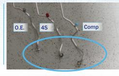
Competitor design does not match the O.E. line design causing the installer to torque the fitting to the condenser, creating stress to the line.
