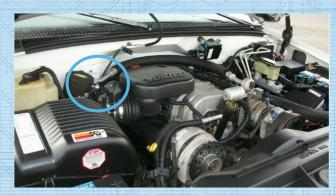
Competitor unit has wrong bend leading to the accumulator. This forces the installer to twist and manipulate the line in order to install on the vehicle, which may cause damage and stress to hose and crimps.
