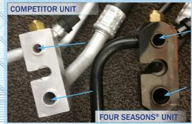
Competitors manifold inner diameter is smaller than the Four Seasons\* and the O.E. unit, restricting oil and refrigerant flow.
