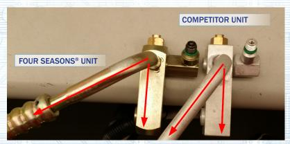
Competitor incorrect angle from the manifold block will cause installer to manipulate line in order to install.
