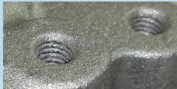
The competitor unit shows signs of sandblasting of the threaded surface. This lack of process control creates a coating that could cause the thread wall to strip, making installation difficult.
