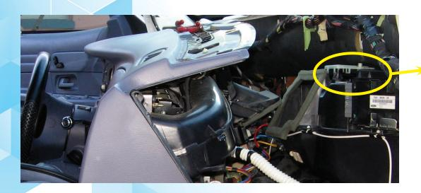
Air door actuator located behind the dash requiring a full removal and up to 8 hours of labor
