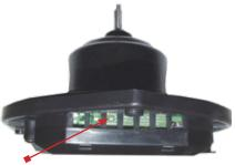
Exposed Traces on Printed Circuit Board (PCB)
