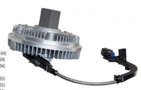
Hayden's manufactured Ford EVC Fan Clutch, part number 3261, impresses customers with it's durability, longevity and quality design. KEVIN ROBERTS OF ROBERTS REPAIR IN RHINELANDER, WISCONSIN, has specialized in emergency vehicle maintenance and repair for nearly 30 years. After repeat O.E. fan clutch failures on the E450 Ford emergency vehicle, Kevin found success switching to Hayden's manufactured unit. Hear why Kevin chooses a trusted supplier and quality parts.
